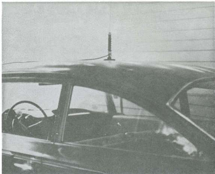
Fig. 7-48. Antenna mounted on top of author's 1960 Chevrolet.
